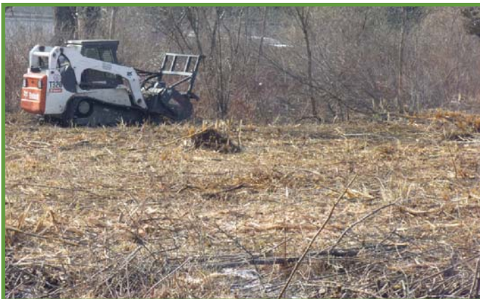
A site in Dutchess County where overgrown vegetation was removed using a skid steer with fecon head attachment. Photo credit: N. Rayman
